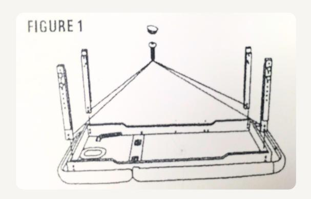
Securely attach the four legs to the four corners of the tabletop using screw #1 along with nut #4 and nut cap #2 on the opposite side, ensuring a tight fit as depicted in the image below.
