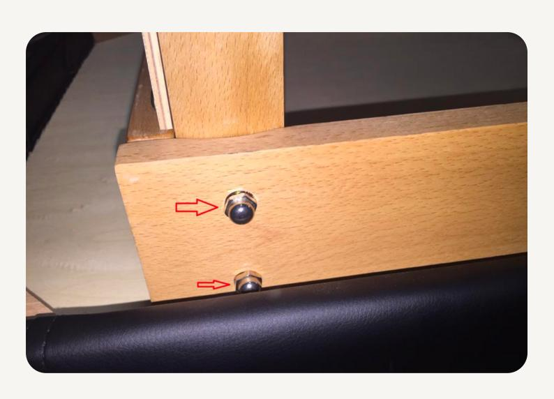
Use the screws #3 to fasten up the pallet board to the four legs for the base of the bed as shown in the image bellow. Make sure they are tightly secure
