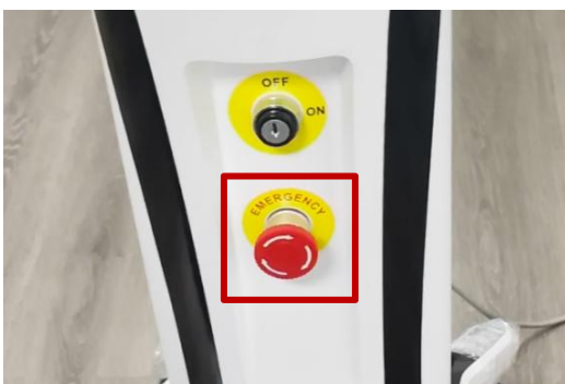
Red emergency switch
